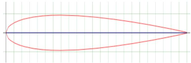
Fig. 4: NACA0008 Airfoil
