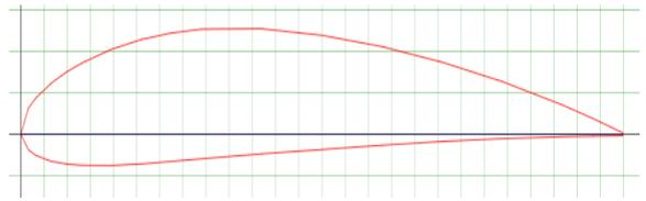
Fig. 3: NACA 4412 Airfoil
