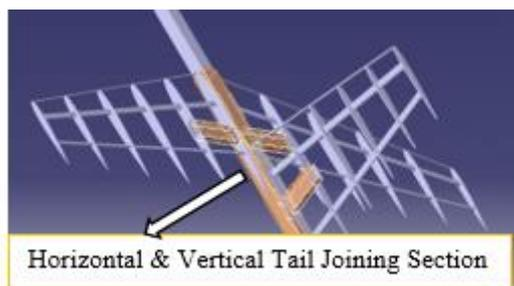
Fig.11: Horizontal and Vertical Tail Section
