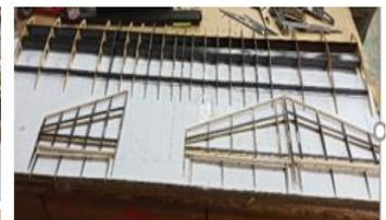
Fig. 24: Horizontal and Vertical tail parts assembly
