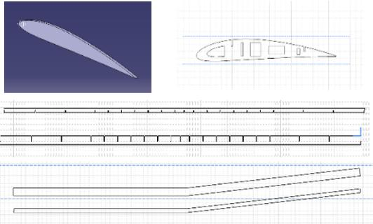
Fig.8: Airfoil, ribs, spars, and dihedral rods
