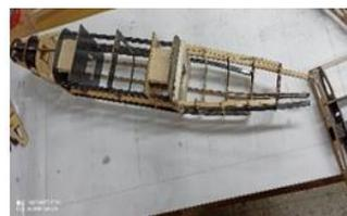
Fig. 25: Fuselage nose section Parts assembly
