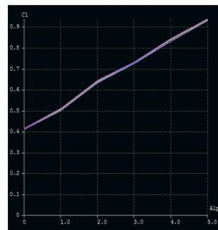
Fig. 5: XFLR analysis graph Cl Vs Alpha
