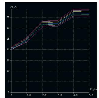
Fig. 6: XFLR analysis graph Cl/Cd Vs Alpha
