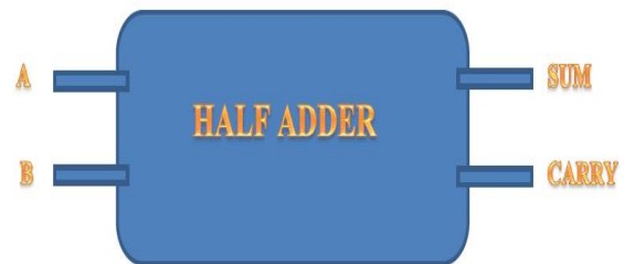
Fig.1 Block diagram for half adder
