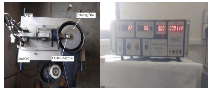
Fig.3. (a) DUCOM Pin on Disk Setup (b) Control Unit
