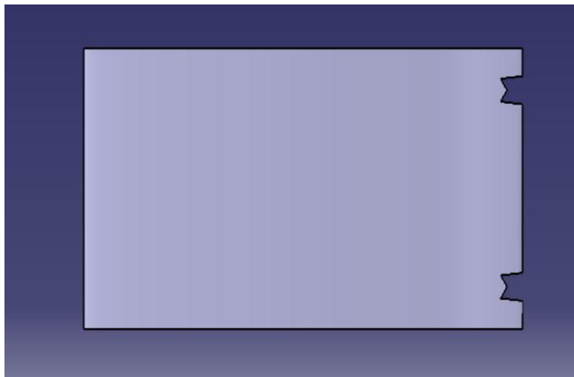
Fig. 1. Stator blade with 'M' cut at tip
