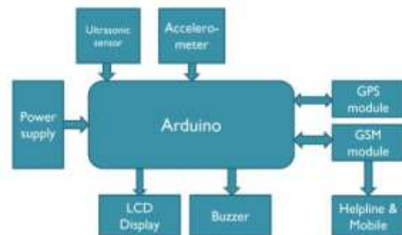
Figure 1 Block diagram of Anti-Collision system using GPS and GSM module
