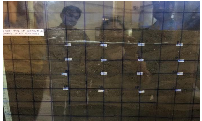
Fig 1. Geometry of the planar geotextile-reinforced foundation bed.
