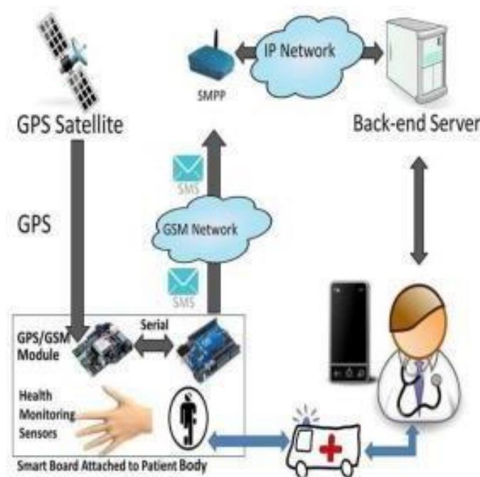
Fig-2 :System Architecture
