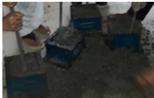
(a) Compaction by using a tamping rod
