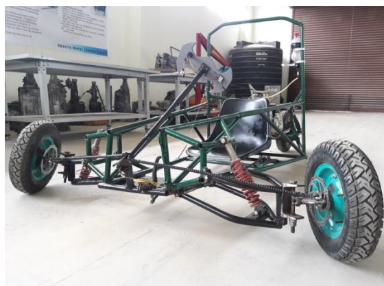
Fig 11. Fabricated Model of Trike
