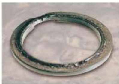
Figure 22 The Cracked Outer Sealing Lip of Wiper Seal which displays Damage caused by Excessive Heat
