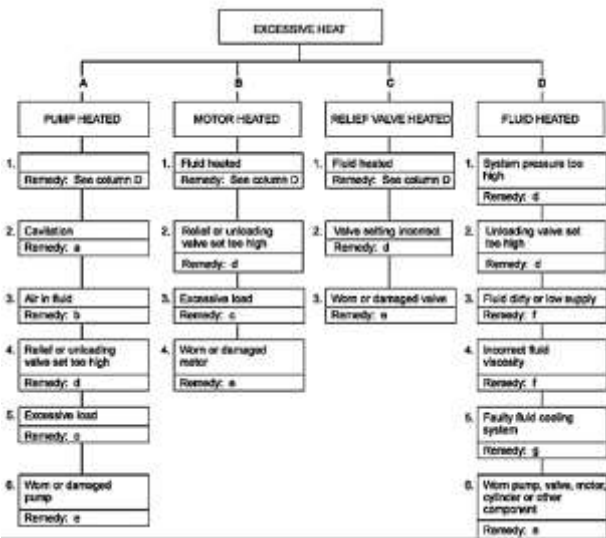
Chart 6.2 the Causes of Excessive Heat
