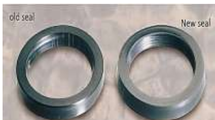
Figure 21 the Contamination Damage in Rod Seal
