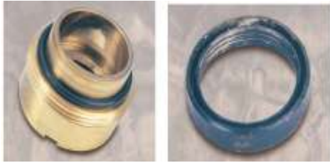
Figure 20 the Wear in Gland and Seal which results from Excessive Side Loading
