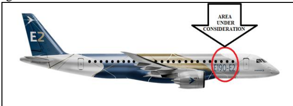
Fig.1. Embraer E190 depicting the area under consideration for drop-test analysis
