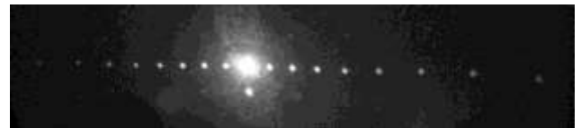
Fig.5. The diffraction orders recorded under Raman-Nath diffraction conditions
