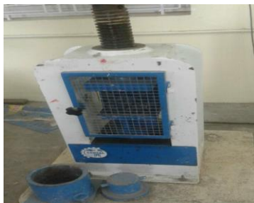
Fig 4 – Test on Compression strength for cubes
