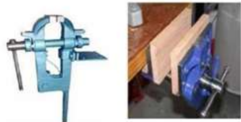
FIG 1.22POST VICE FIG 1.23WOODWORKVICE
