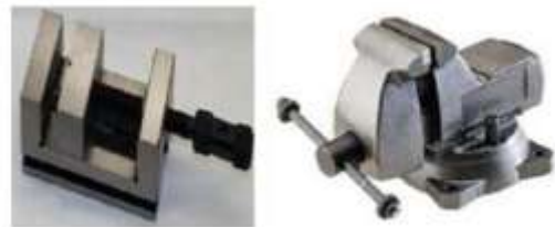
FIG1.2 MACHINIST VICE FIG1.21MECHANICVICE
