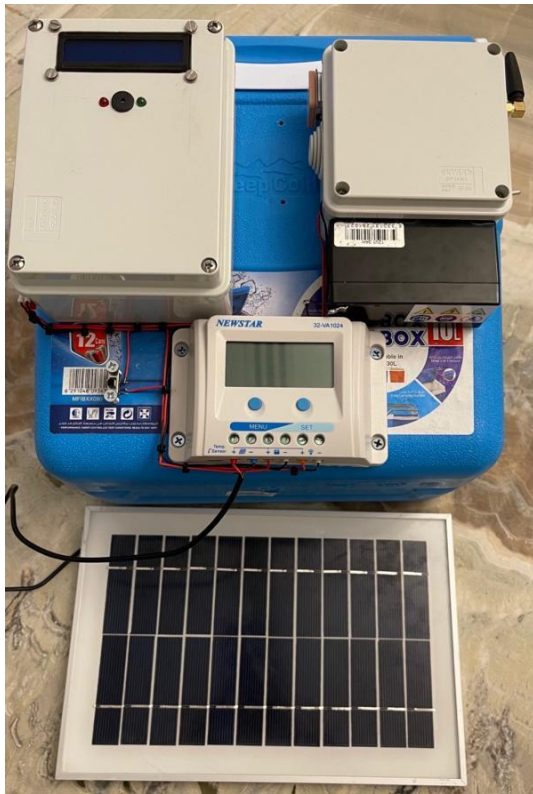
Fig. 15. Temperature Monitoring and Tracking Vaccine Box
