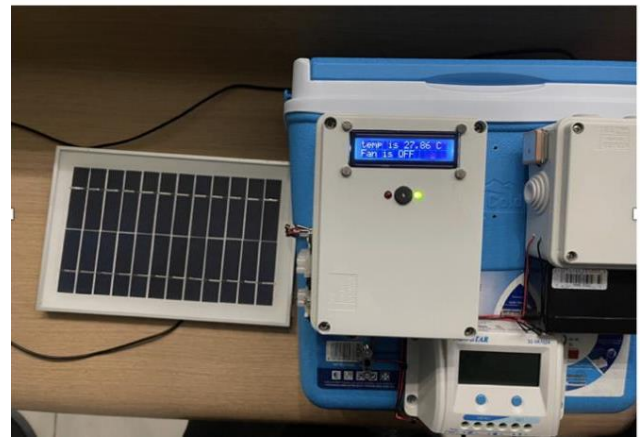
Fig.13. Temperature Monitoring System
