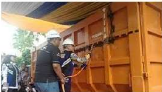
Fig.2. ODOL Truck Controlled Body Cutting During Department of Transportation Control(12).
