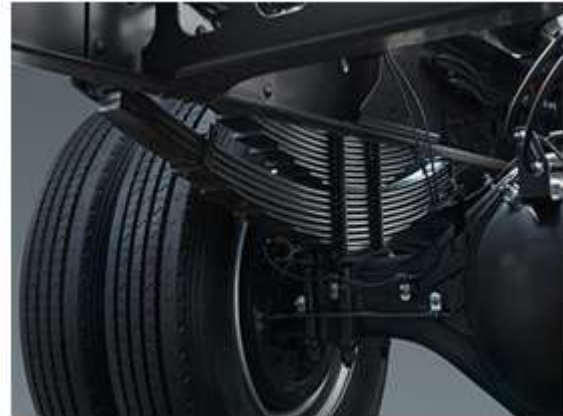
Fig. 4. Main Leaf Spring and Helper Spring on Hino 500 Fg260 (21)
