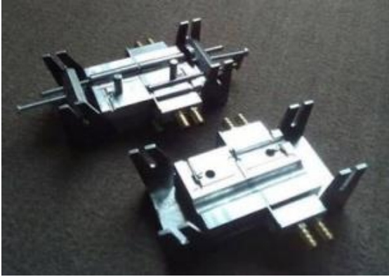
Photographs of the injection molds of the collecting discs and the links
