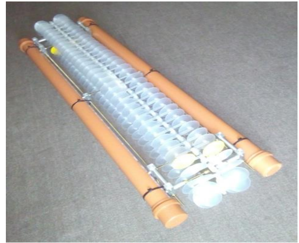
1 meter in length prototype with 72 polypropylene links and their discs and side floats ( N = 30 )
