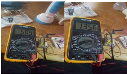
Fig. 17. Rectified LM7805 Input and output Voltage (Breadboard)
