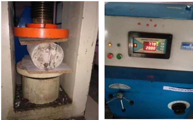
Fig-3: Testing of cylinders
