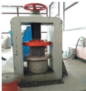
Fig-1: testing of cube specimen
