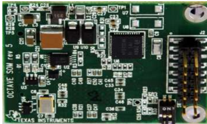
Fig. 2: SOMPLC-F28PLC83System on Module for Power Line Communication
