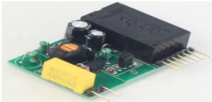
Fig.4. KQ-130F power line carrier data transceiver module
