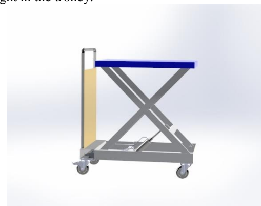
Fig. 8. Image of newly designed Hydraulic Trolley
