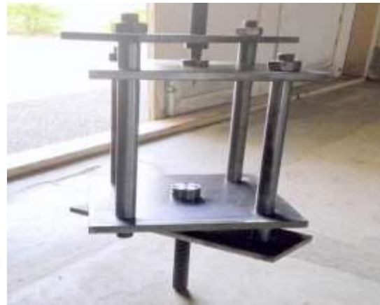
Figure 3.5 Small punch test fixture with specimen holder, punch holder, punch & connecting rods in an assembled mode.
