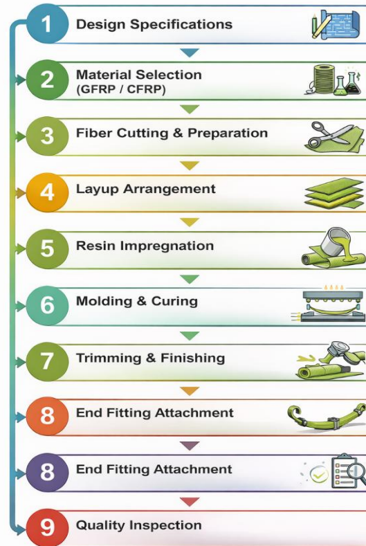
Figure.2: Step-By-Step Fabrication Flow Chart
