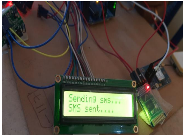
Figure11. It shows that when the woman is in the danger mode any sensor detects the women tracking location and sends the SMS.
