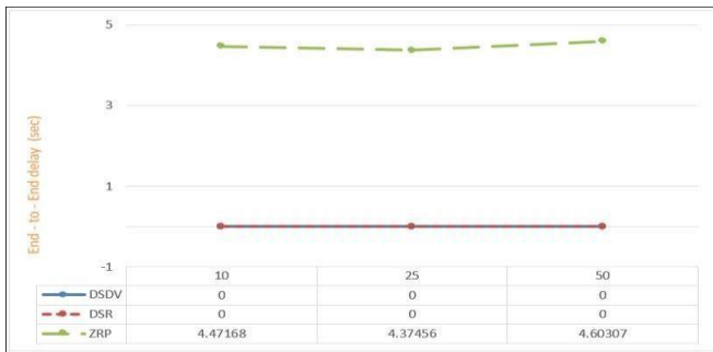
Figure 8. E2E delay vs. Number of Nodes 100 pause time
