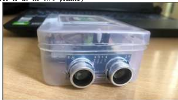
Fig. 3 Device containing Ultrasonic Sensor
