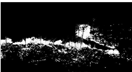
Fig. 7. The processed image on the Django web-app after applying the Sobel edge detection algorithm.
