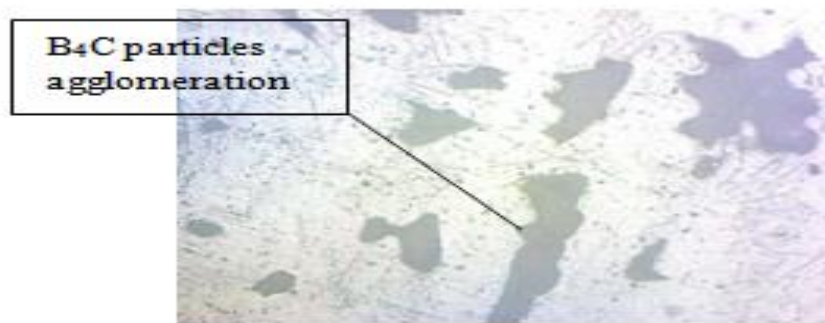
Figure 7 Optical micrograph of a composite
