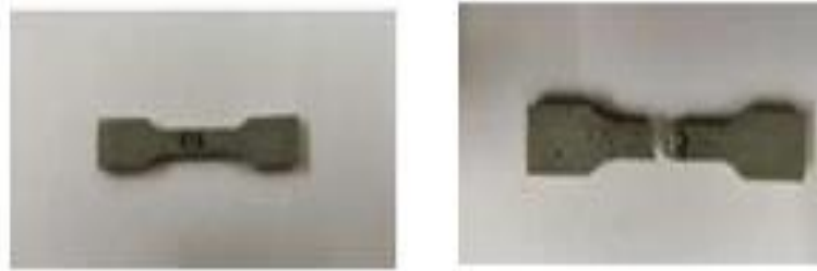
Figure 13 AMC MS-200 specimens-Before and after tensile test
