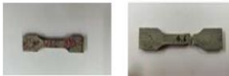
Figure 14 AMC MS-270 specimen-Before and after tensile test
