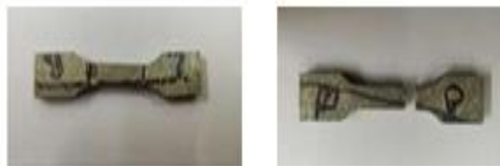
Figure 12 AMC MS-150 specimens-Before and after tensile test
