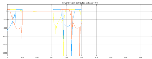
Fig 2. Three phase voltages when DSTATCOM is not connected to transmission lines and fault is introduced
