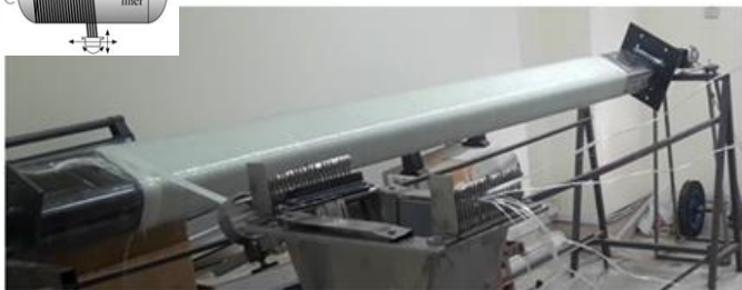
Fig. 1. Circumferential pattern of winding [90°]
