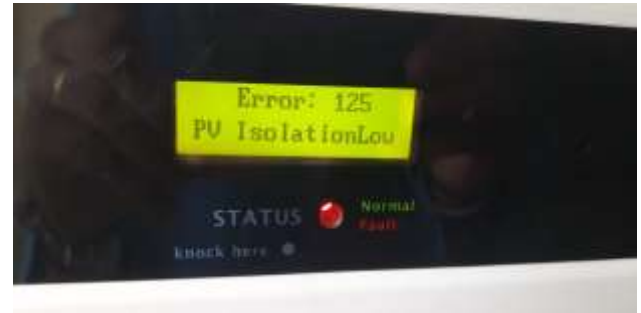
Figure 7: Error: 125 display on the inverter screen
