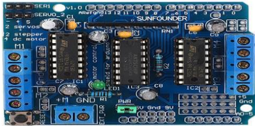
Fig 2.3 - Motor driver L293D
