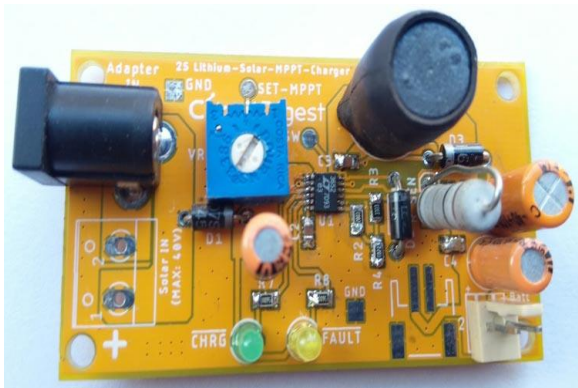
Fig 5 MPPT Charge controller
