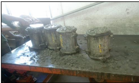
Fig .4.Casting Of Cylinder
