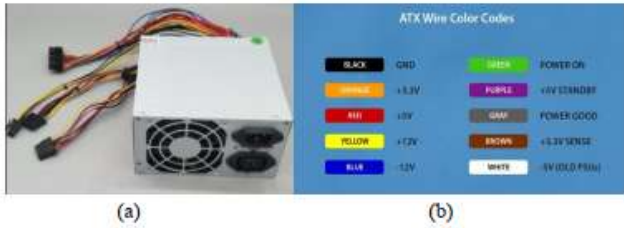
Fig. 12. (a) ATX power supply (b) ATX color code
