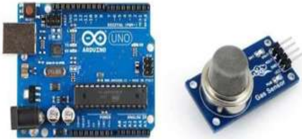
Figure1. Arduino UNO microcontroller and MQ-6 Sensor
