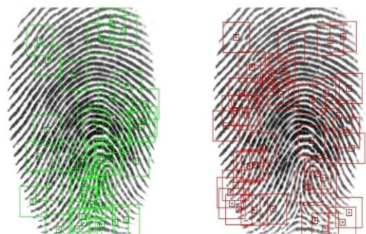
Figure(B):50*50 patches with non-minutiae patches that do not contain any minutiae points at 10*10 center
