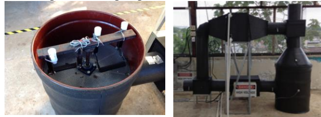
Figure 1: Photographs of the parchment coffee dehydration prototype systems. Left: open rotary drum dryer referred to as the opened-batea (OB) configuration. Right: HARC 2 S referred to as the closed-batea (CB) configuration. The top middle component is the HX that removes dehydration water from the thermodynamic cycle.
