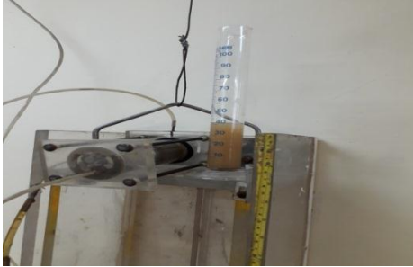
Fig. 8. Heavy Colloidal discharge at 50mm head in pin hole test
