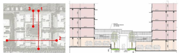
Figure 15 : Key Plan and Section 3: Detail of green connect between parking levels Source: Author
