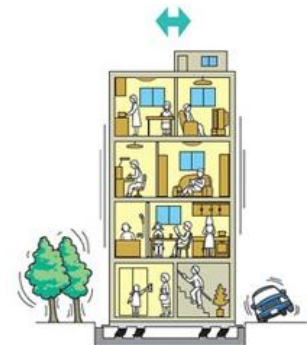
Fig. 2: Base isolated building ( https://www.kuraka.co.jp/en/technology )
