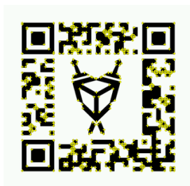
Fig. 5. Feature point detection using Vuforia Engine.
