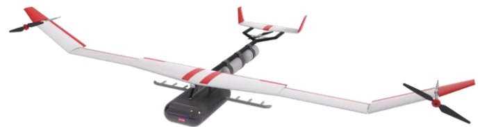
Fig. 14. Rendered Image of High Altitude, High Stability Flight Mode attached with a Module
