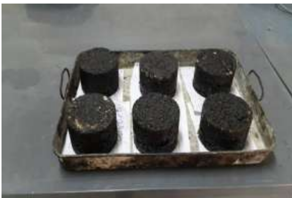
Fig. 1. Marshal Molds at different percentages of bitumen
