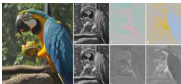
Fig 3.7 Lightness, *a, and *b channels of Lab color space for an image | Image from Rodrigo Berriel
