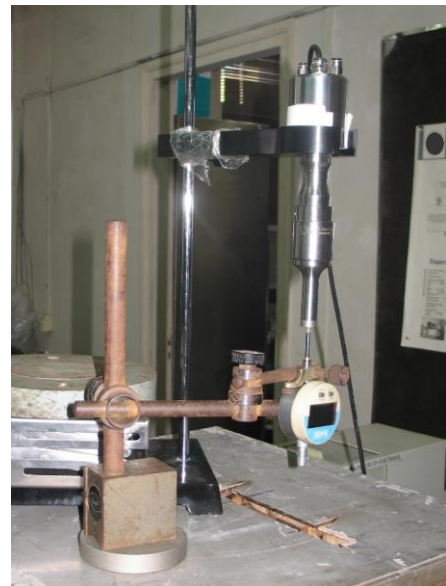
Fig. 3. Calibration by Digital Dial Indicator
