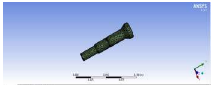
Fig. 3. Meshing of Punch Model Modified (3)
