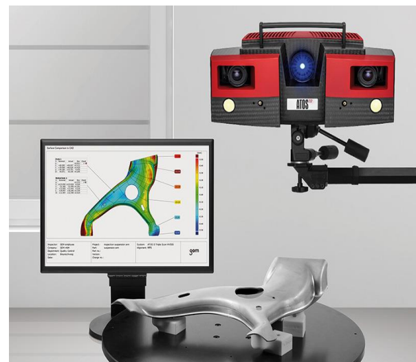
Fig. 3D Scanning of component
