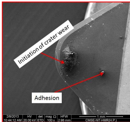
Fig. 5. Interrupt machining at 102 m/min and and 20 passes
