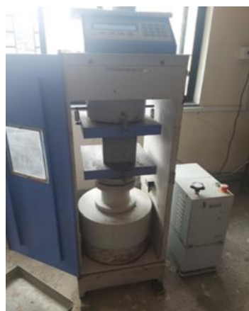
Fig -1 : Testing of Concrete cubes
